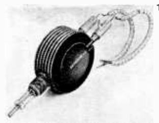
Air-cooled Magnetron valve made by M.O. Valve Company. A pulse output of 450 kW is given at centimetric wavelengths.
